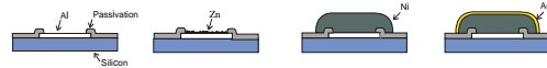
Figure 2: Principle process of electroless Ni bumping: (a) bondpad in initial state, (b) after zinc deposition, (c) after growth of electroless Ni, (d) after plating of thin immersion Au.
